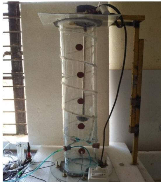
Figure 3.10. Experimental setup of the Continuous Column Used for Adsorption Study
