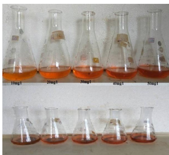
Figure.4.29. Removal of RO onto CPPA at Optimized Condition
