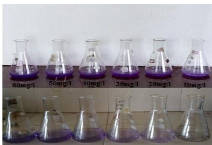
Figure 4.20. Removal of CV onto CP at Optimized Condition
