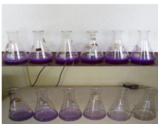
Figure.4.23 Removal of CV onto CPPA at Optimized Condition
